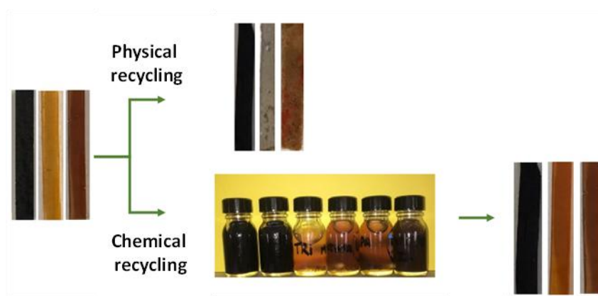
Fig. 1: Chemical and mechanical recycling of epoxy-anhydride networks
